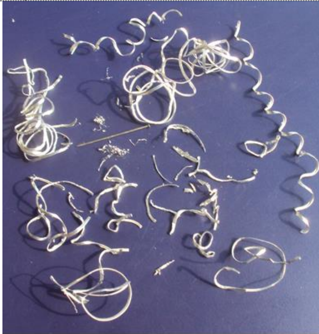
Figure 2. Resulted chips after turning with a feed f=0.096 mm/rot.
